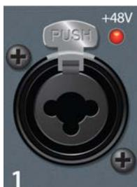
**Mic/Line Inputs.** The inputs on your NSB-Stagebox can also accept mic- or line-level signals. These inputs use TRS-XLR combo jacks that can accept both XLR and balanced or unbalanced 1/4" cables.
