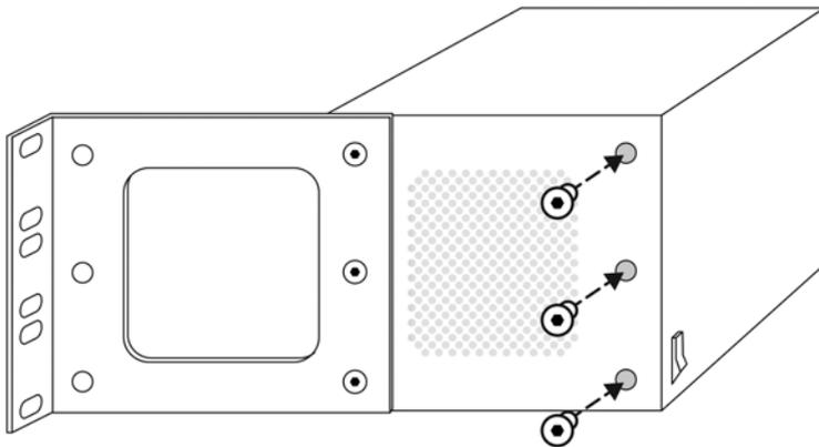
For a reversed configuration, simply rotate the ears 180° and re-attach the screws.
