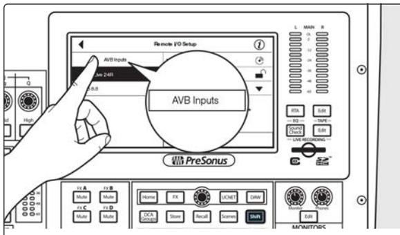
On the Remote I/O screen, press AVB Inputs.
