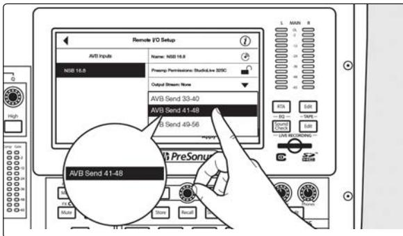
Select the AVB Output Sends you'd like returned to the physical outputs on your NSB stage box. Because the AVB streams must be routed in banks of 8, you can only source these outputs from one mixer on the network.
