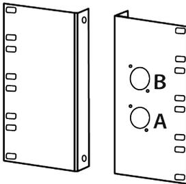
**NSB 16.8 or NSB 8.8 Rack adapter.** PreSonus has designed the NSB 16.8 and NSB 8.8 adapters to mount the NSB-series stage boxes in standard 19" equipment rack. This accessory is sold separately at your favorite PreSonus dealer or at [www.presonus.com](http://www.presonus.com).
