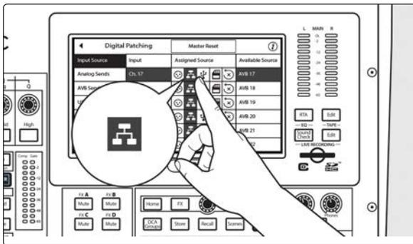
Scroll to Inputs 9-32 and assign each to the Network source by pressing the Network button next to each Input.
