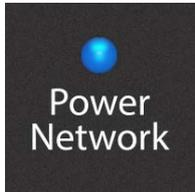
The Power Network LED on your NSB stage box will turn from green to blue when proper clock sync has been established with the AVB network.
