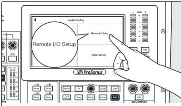
Press the Remote I/O Setup button on the Touchscreen.
