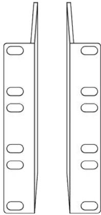
**Reversible Rack Ears (NSB 32.16 only)** The rack ears included with the NSB 32.16 are reversible, allowing the mixer to be racked in either recessed or reversed configurations, allowing space for all attached cabling when installing NSB 32.16 in a stage rack.
