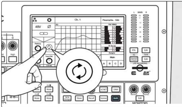
After you have set the preamp levels, enable Gain Compensation from the LCD. This will turn on Gain Compensation for that input and allow other mixers on the network to source that stream.
