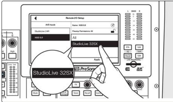
The preamps on NSB-series stage boxes can be controlled from any StudioLive Series III mixer on the network. When you have a stage box feeding more than one mixer, it is recommended that you give only one mixer permission to adjust the NSB preamp levels. In our example, we will be giving permission to the StudioLive 32SX at Front-of-House.
