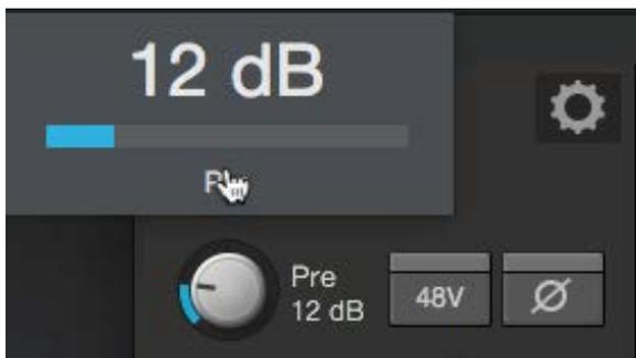
You can now control the preamp level and phantom power for your NSB stage box from the Fat Channel in Universal Control, in the same way that you control the local inputs.
