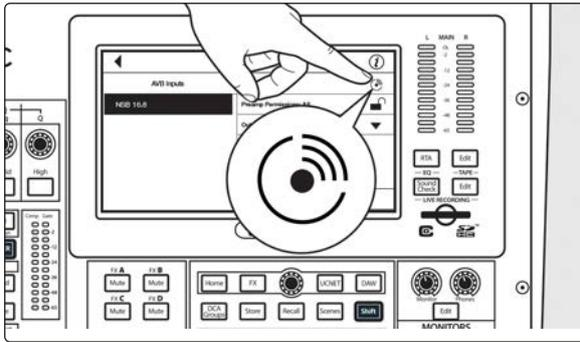
In applications where you are using multiple NSB-series stage boxes of the same model, you can press the Identify button. This will flash the Power Network LED on the front of the selected NSB stage box from green to red, allowing you to quickly locate your selection.
