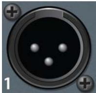
**Line Out.** These balanced XLR line outputs are to connect external devices like powered floor monitors, amplifiers, etc.
