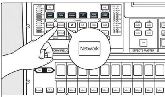
The Network Source can also be enabled for each channel individually from the Fat Channel. Using the Digital Patching screen allows you to assign the sources to multiple channels at once. Your NSB 8.8 is now ready to use with your StudioLive 32SX. Now let's set it up for the StudioLive 24R!
