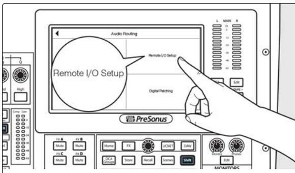
Press the Remote I/O button on the Touch-screen.
