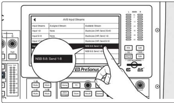
When using a StudioLive Series III console as the master preamp controller for your NSB-series stage box, select the non-Gain Compensated streams for your inputs.
