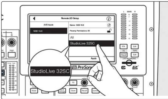
Select the mixer you'd like to use to control the preamps on your NSB stage box. By default, this is set to "All", enabling any StudioLive Series III mixer on the AVB network to control the preamps on your stage box.
