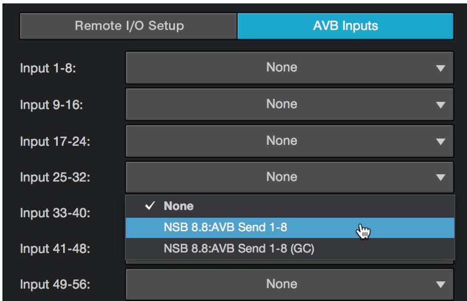
**Power User Tip:** NSB stage boxes have two sets of streams: one with Gain Compensation and one without. In our example, the StudioLive 24R has total preamp control over the NSB stage box and is the only mixer connect to its streams, because of this, Gain Compensation is not required in this example. Please review [the Gain](#)
