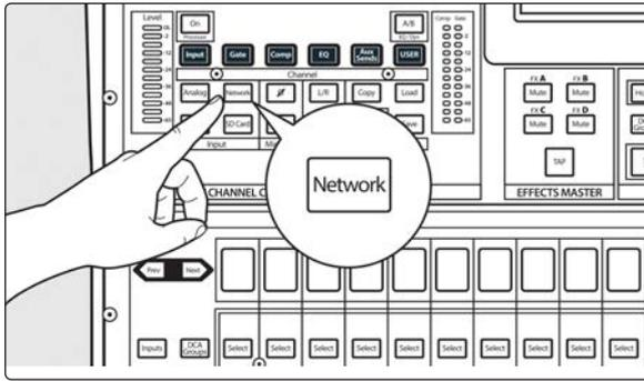
Select each channel and press the Network button from the Input source section in the Fat Channel. **Your NSB 16.8 is now ready to use!**
