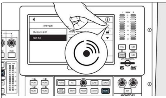
In applications where you are using multiple NSB-series stage boxes of the same model, you can press the Identify button. This will flash Power / Network LED on the top panel red and green on the currently selected NSB, allowing you to quickly locate your selection.
