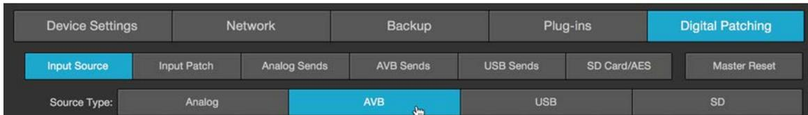
3. Click or tap on the source icon for Channels 25-32 to change each channel's source input to AVB. This will enable the corresponding NSB stage box input to each channel (e.g. NSB Input 1 will be enabled on StudioLive 24R channel 25, NSB Input 2 will be enabled on StudioLive 24R channel 26, etc.)
