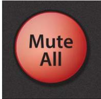
**Mute All.** This button mutes every input and output on your NSB. Use this button to quickly silence your NSB while making connections or disconnecting equipment to avoid volume spikes in your system.
