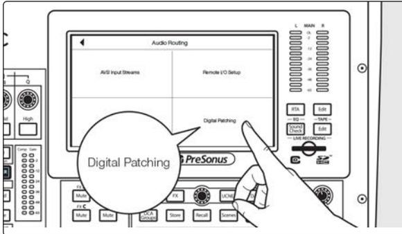
Press the Digital Patching button to open the Digital Patching screen.
