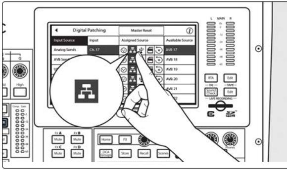
Select Input Source and scroll to Inputs 17-32. Assign each to the Network source by pressing the Network button next to each Input. Or....
