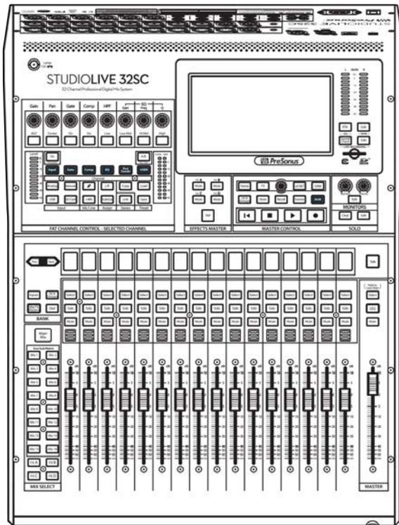
**1722.1 AVB-compatible mixer.** All PreSonus StudioLive Series III mixer models are fully compatible with the 1722.1 AVB standard and NSB-series stage boxes. If you are using a third-party AVB mixer, please contact the manufacturer to verify compatibility with this standard.
