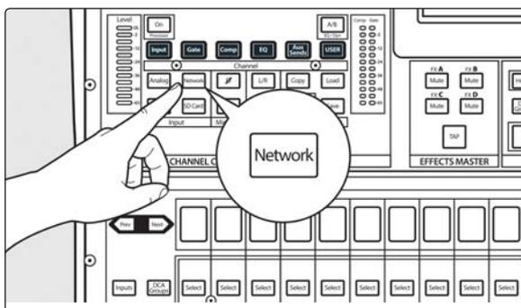
After you route the NSB inputs to your console mixer, select Network for the source on the corresponding channels.
