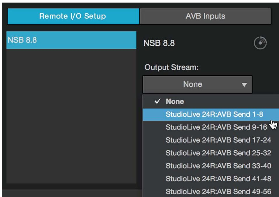
**Note:** You must assign an output stream from your mixer to your NSB-series stage box so that it is clocked properly over the network. If you do not assign an output stream from your mixer, your networked
