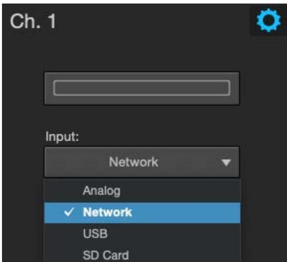
After you route the NSB inputs to your console mixer, select Network for the source on the corresponding channels.
