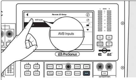
In our example, we are using the NSB 16.8 to add 16 additional analog inputs and 8 additional analog outputs to a StudioLive 32SC. Press the AVB Inputs button.
